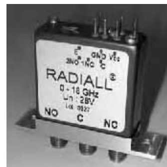
A SMA SPDT with a specific RF body (with mounting leg) for easy mounting on front panel of switching matrix.
