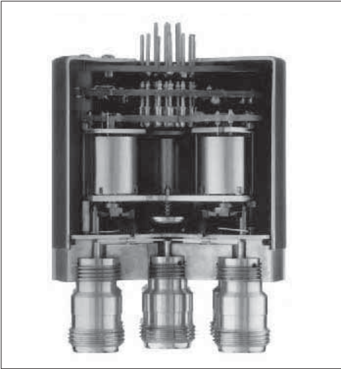
Figure 2 : A Cutaway view of RAMSES coaxial switch
